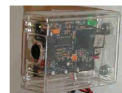
Infrared sensors When visitors cut infrared by to pass between infrared sensors, a bulb conected with sensor is turned on and after 4 sec. it is turned off automatically
